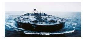
Tankers can appear similar to bulk carriers, but the deck is flush and covered by oil pipelines and vents. Tankers transport petroleum products, chemicals and crude oil.
